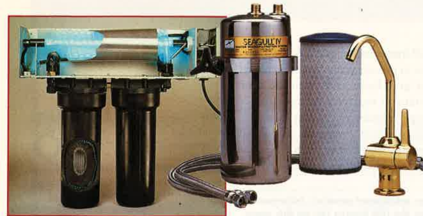
The Ster-L-Tech Life Flo filter (left) combines an activated-carbon filter with a disinfecting UV light. General Ecology's Seagull IV system (right) uses submicron filtration to remove bacteria, sediment and some toxic chemicals.
